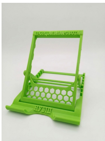
Fig. 2. A mobile phone stand produced using 3D printing technology
